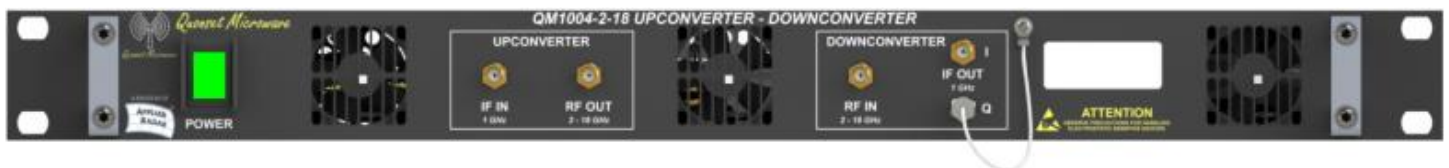
Figure 2. Front panel connections to QM1004-0.5-18.
