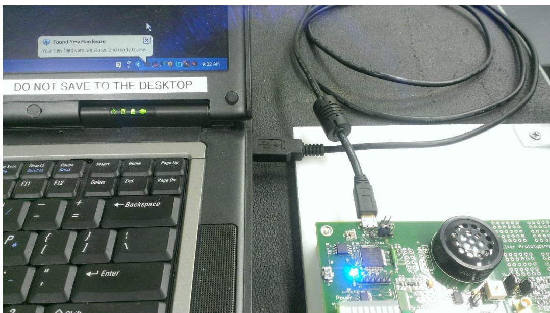
Figure 3: RDK Connected to Laptop Using a USB Cable
