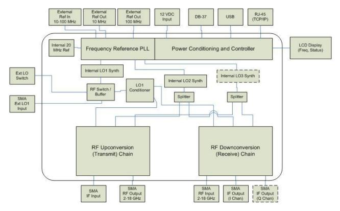
Figure 1. QM1004-8-12 block diagram for the Base System (Option 100) with optional third LO for optional third conversion stage (Options 200 or 201) shown in dashed line.
