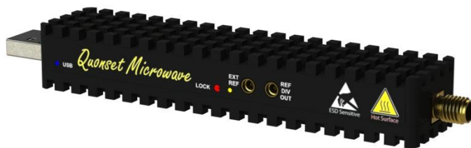
QM2010-24-27 Side View USB, Lock Status, and External Reference LEDs External Reference MMCX input, Reference Out MMCX output
