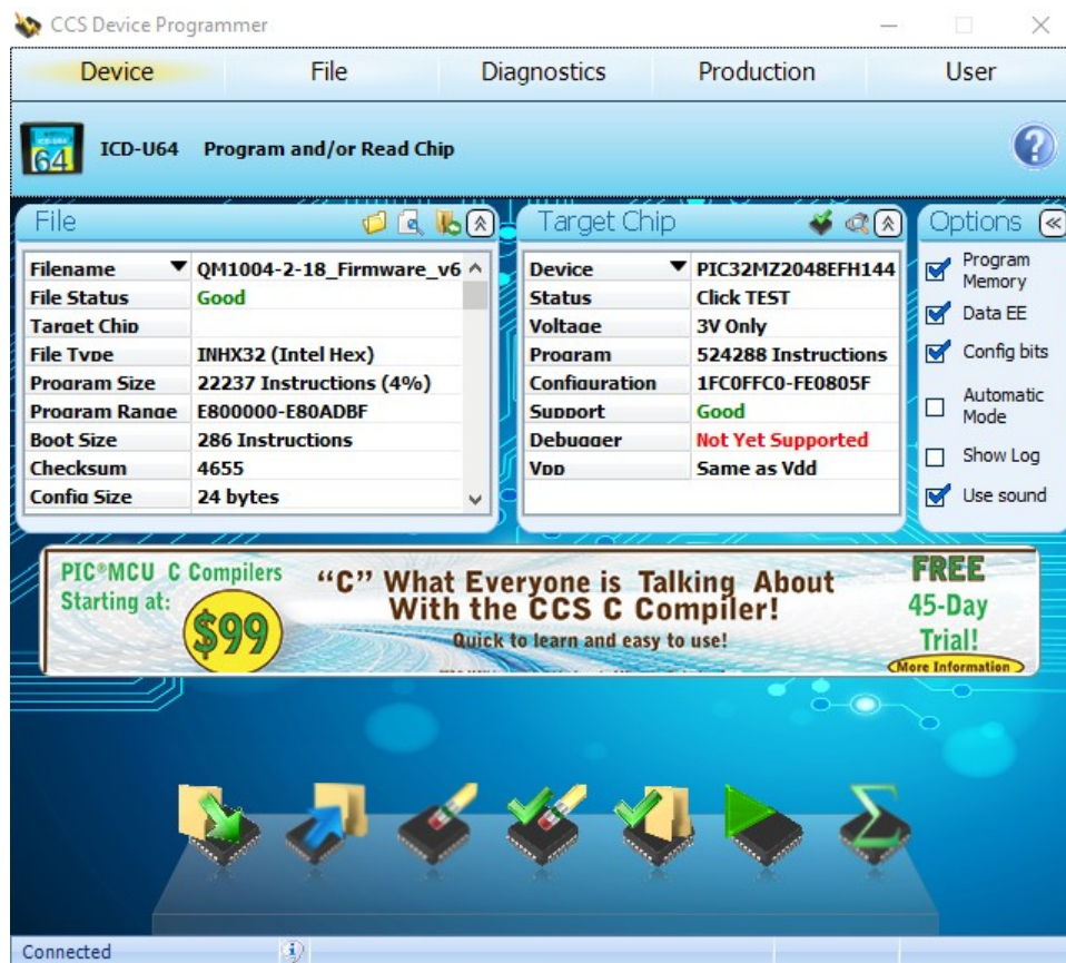
Figure 2.12: CCSLOAD: PIC Programming
