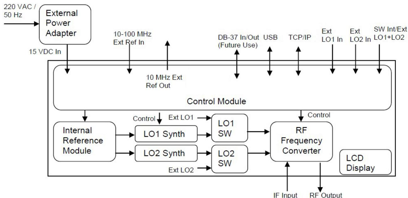
**Figure 1.2:** QM1013–101 Upconverter Block Diagram
