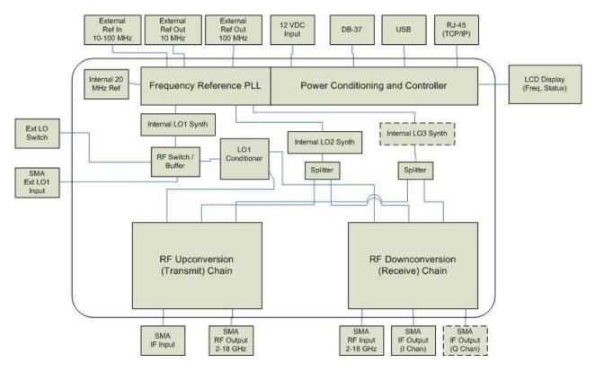
Figure 1. QM1004-2-18 block diagram for the Base System (Option 100) with optional third LO for optional third conversion stage (Options 200 or 201) shown in dashed line.
